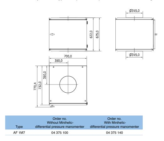
Cabinet for absolute filter type AF1 (excl. filter) on legs with connection in through side and out of top:
