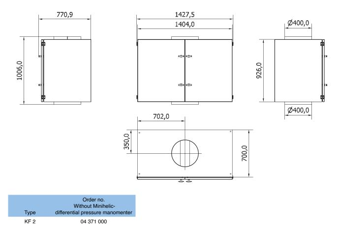
Cabinet for compact filter type AF1 (excl. filters) with connection in through bottom and out of top:
