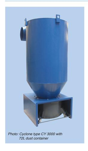
As coarse separator before filter units or as fan protection you can advantageously use a cyclone of the type CY. For high vacuum the model CY-V can be used and for pre-separation of light materials the LCY with high separation/low rise velocity is recommended.
