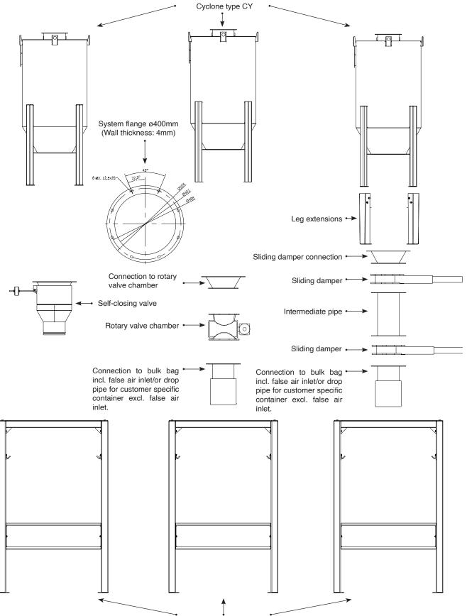
Underframe for suspension of bulk bag or insertion of customer specific container.
