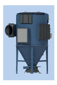
Energy-optimized unit for larger filtration tasks, where there is a dust explosion risk, e.g. at filtration of aluminium dust, wood dust or dust from various powder mix handlings. Unit is constructed for application at ATEX-zones 21-22 and is standard equipped with relief membrane, designed to break at an explosion, whereby the unit is relieved and explosions controlled.
