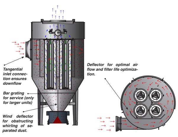
Cyclone filter type ACF/ACF-T/ACF-V is constructed according to:
