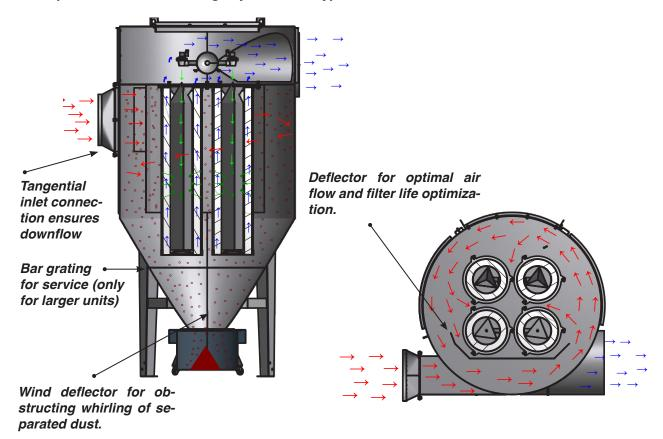
Principle sketch for flow through cyclone filter type ACF-T:
