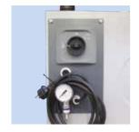
Motor protection/ compressed-air Integrated motor protection and easy access for compressedair connection by cejn-coupling. Pressure tank in unit. Filter cleaning activated by push button.
