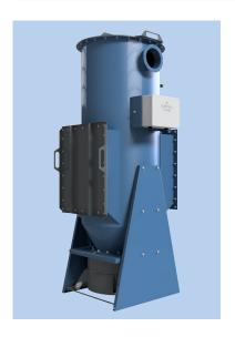
Compact compressed-air cleaned filter unit for smaller filtering tasks, where there is a dust explosion risk, e.g. at filtration of metal dust, wood dust or dust from various powder mix handlings. Unit is constructed for application at ATEX-zones 21-22 and is standard equipped with relief membrane, designed to break at an explosion, whereby the unit is relieved and explosions controlled.
