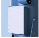
Relief membrane Relief membrane on the back. placed Be aware of pressure wave and flame spread  $\aleph$ through it at relief of a & possible dust explosion.
